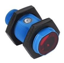
Contrinex photoelectric sensor, tubular, threaded, ABS plastic housing, through-beam receiver, 0-30m sensing distance, 10-30 VDC operating voltage, complementary light-on/dark-on, NPN, 4-wire, 4-pin M12 quick-disconnect.
