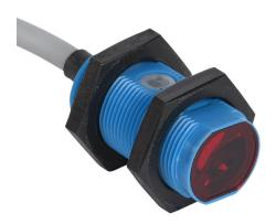
Contrinex photoelectric sensor, tubular, threaded, ABS plastic housing, through-beam emitter, visible red, 0-30m sensing distance, 10-30 VDC operating voltage, 3-wire, pigtail.
