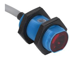
Contrinex photoelectric sensor, tubular, threaded, ABS plastic housing, through-beam emitter, visible red light emission, 0-30m sensing distance, 10-30 VDC operating voltage, 3-wire, pigtail.
