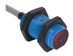
Contrinex photoelectric sensor, tubular, threaded, ABS plastic housing, through-beam receiver, 0-30m sensing distance, 10-30 VDC operating voltage, complementary light-on/dark-on, NPN, 4-wire, pigtail.
