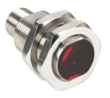
Contrinex photoelectric sensor, tubular, threaded, stainless steel housing, through-beam receiver, 0-30m sensing distance, 10-30 VDC operating voltage, complementary light-on/dark-on, PNP, 4-wire, 4-pin M12 quick-disconnect.
