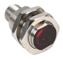
Contrinex photoelectric sensor, tubular, threaded, stainless steel housing, through-beam emitter, visible red, 0-30m sensing distance, 10-30 VDC operating voltage, 3-wire, 4-pin M12 quick-disconnect.
