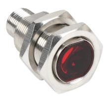
Contrinex photoelectric sensor, tubular, threaded, stainless steel housing, through-beam receiver, 0-30m sensing distance, 10-30 VDC operating voltage, complementary light-on/dark-on, NPN, 4-wire, 4-pin M12 quick-disconnect.
