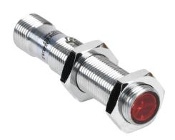
Contrinex photoelectric sensor, tubular, threaded, chrome-plated brass housing, through-beam receiver, 0-10m sensing distance, 10-30 VDC operating voltage, complementary light-on/dark-on, PNP, 4-wire, 4-pin M12 quick-disconnect.
