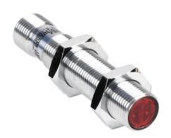
Contrinex photoelectric sensor, tubular, threaded, chrome-plated brass housing, through-beam emitter, visible red, 0-10m sensing distance, 10-30 VDC operating voltage, 3-wire, 4-pin M12 quick-disconnect.
