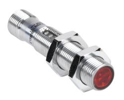
Contrinex photoelectric sensor, tubular, threaded, chrome-plated brass housing, through-beam receiver, 0-10m sensing distance, 10-30 VDC operating voltage, complementary light-on/dark-on, NPN, 4-wire, 4-pin M12 quick-disconnect.
