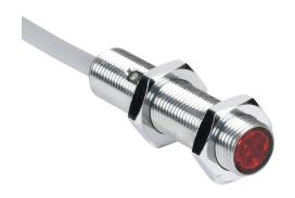
Contrinex photoelectric sensor, tubular, threaded, chrome-plated brass housing, through-beam receiver, 0-10m sensing distance, 10-30 VDC operating voltage, complementary light-on/dark-on, PNP, 4-wire, pigtail.
