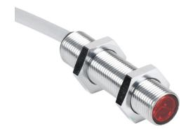
Contrinex photoelectric sensor, tubular, threaded, chrome-plated brass housing, through-beam emitter, visible red light emission, 0-10m sensing distance, 10-30 VDC operating voltage, 3-wire, pigtail.
