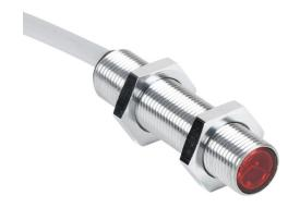
Contrinex photoelectric sensor, tubular, threaded, chrome-plated brass housing, through-beam emitter, visible red, 0-10m sensing distance, 10-30 VDC operating voltage, 3-wire, pigtail.
