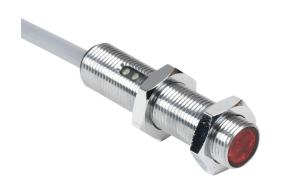
Contrinex photoelectric sensor, tubular, threaded, chrome-plated brass housing, through-beam receiver, 0-10m sensing distance, 10-30 VDC operating voltage, complementary light-on/dark-on, NPN, 4-wire, pigtail.
