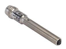
Contrinex photoelectric sensor, tubular, threaded, stainless steel housing, through-beam receiver, 0-600mm sensing distance, 10-30 VDC operating voltage, dark-on, PNP, 3-wire, 3-pin M8 quick-disconnect.
