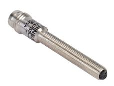
Contrinex photoelectric sensor, tubular, threaded, stainless steel housing, through-beam emitter, visible red light emission, 0-600mm sensing distance, 10-30 VDC operating voltage, 3-wire, 3-pin M8 quick-disconnect.
