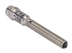
Contrinex photoelectric sensor, tubular, threaded, stainless steel housing, through-beam receiver, 0-600mm sensing distance, 10-30 VDC operating voltage, dark-on, NPN, 3-wire, 3-pin M8 quick-disconnect.
