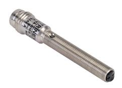
Contrinex photoelectric sensor, tubular, threaded, stainless steel housing, through-beam receiver, 0-600mm sensing distance, 10-30 VDC operating voltage, dark-on, NPN, 3-wire, 3-pin M8 quick-disconnect.
