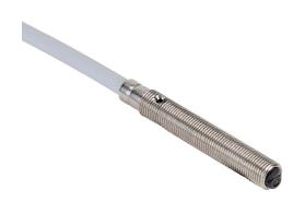
Contrinex photoelectric sensor, tubular, threaded, stainless steel housing, through-beam receiver, 0-600mm sensing distance, 10-30 VDC operating voltage, dark-on, PNP, 3-wire, pigtail.
