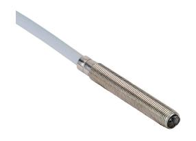
Contrinex photoelectric sensor, tubular, threaded, stainless steel housing, through-beam emitter, visible red, 0-600mm sensing distance, 10-30 VDC operating voltage, 3-wire, pigtail.
