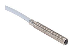
Contrinex photoelectric sensor, tubular, threaded, stainless steel housing, through-beam receiver, 0-600mm sensing distance, 10-30 VDC operating voltage, dark-on, NPN, 3-wire, pigtail.
