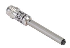
Contrinex photoelectric sensor, tubular, smooth, stainless steel housing, through-beam receiver, 0-600mm sensing distance, 10-30 VDC operating voltage, dark-on, PNP, 3-wire, 3-pin M8 quick-disconnect.
