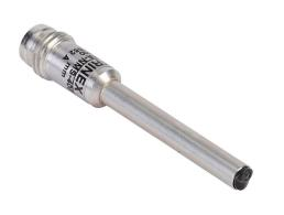
Contrinex photoelectric sensor, tubular, smooth, stainless steel housing, through-beam emitter, visible red, 0-600mm sensing distance, 10-30 VDC operating voltage, 3-wire, 3-pin M8 quick-disconnect.
