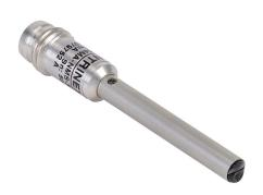
Contrinex photoelectric sensor, tubular, smooth, stainless steel housing, through-beam receiver, 0-600mm sensing distance, 10-30 VDC operating voltage, dark-on, NPN, 3-wire, 3-pin M8 quick-disconnect.
