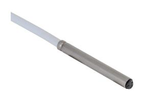
Contrinex photoelectric sensor, tubular, smooth, stainless steel housing, through-beam emitter, visible red, 0-600mm sensing distance, 10-30 VDC operating voltage, 3-wire, pigtail.
