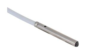
Contrinex photoelectric sensor, tubular, smooth, stainless steel housing, through-beam receiver, 0-600mm sensing distance, 10-30 VDC operating voltage, dark-on, NPN, 3-wire, pigtail.
