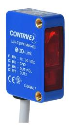
Contrinex photoelectric sensor, rectangular, ABS plastic housing, through-beam receiver, 25m sensing distance, 10-30 VDC operating voltage, complementary light-on/dark-on, PNP, 4-wire, pigtail.
