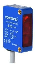
Contrinex photoelectric sensor, rectangular, ABS plastic housing, through-beam receiver, visible red light emission, 25m sensing distance, 10-30 VDC operating voltage, complementary light-on/dark-on, PNP, 4-wire, pigtail.
