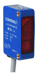
Contrinex photoelectric sensor, rectangular, ABS plastic housing, through-beam emitter, visible red, 25m sensing distance, 10-30 VDC operating voltage, 3-wire, pigtail.
