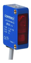
Contrinex photoelectric sensor, rectangular, ABS plastic housing, through-beam emitter, visible red light emission, 25m sensing distance, 10-30 VDC operating voltage, 3-wire, pigtail.
