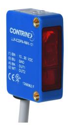
Contrinex photoelectric sensor, rectangular, ABS plastic housing, through-beam receiver, visible red light emission, 25m sensing distance, 10-30 VDC operating voltage, complementary light-on/dark-on, NPN, 4-wire, pigtail.
