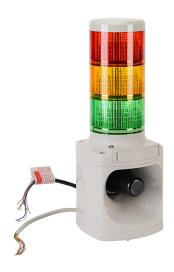
Patlite LED signal tower, (3) tiers, 100mm diameter, red/amber/green, permanent or flashing (60 fpm +/- 3 fpm) light function, (32) alarms, 24 VDC, NPN polarity, colored lens, 385.4mm body length, light gray, 360 degree viewing angle, direct mount, IP53.
