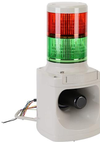
Patlite LED signal tower, (2) tiers, 100mm diameter, red/green, permanent or flashing (60 fpm +/- 3 fpm) light function, (32) alarms, 24 VDC, NPN polarity, colored lens, 325.3mm body length, light gray, 360 degree viewing angle, direct mount, IP53.
