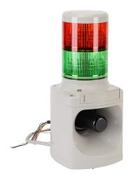
Patlite LED signal tower, (2) tiers, 100mm diameter, red/green, permanent or flashing (60 fpm +/- 3 fpm) light function, (32) alarms, 24 VDC, NPN polarity, colored lens, 325.3mm body length, light gray, 360 degree viewing angle, direct mount, IP53.
