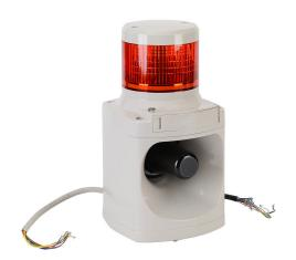
Patlite LED signal tower, (1) tier, 100mm diameter, red, permanent or flashing (60 fpm +/- 3 fpm) light function, (32) alarms, 24 VDC, NPN polarity, colored lens, 265.2mm body length, light gray, 360 degree viewing angle, direct mount, IP53.
