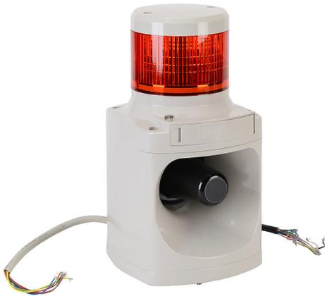
Patlite LED signal tower, (1) tier, 100mm diameter, red, permanent or flashing (60 fpm +/- 3 fpm) light function, (32) alarms, 24 VDC, NPN polarity, colored lens, 265.2mm body length, light gray, 360 degree viewing angle, direct mount, IP53.
