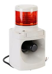
Patlite LED signal tower, (1) tier, 100mm diameter, red, permanent or flashing (60 fpm +/- 3 fpm) light function, (32) alarms, 24 VDC, PNP polarity, colored lens, 265.2mm body length, light gray, 360 degree viewing angle, direct mount, IP53.
