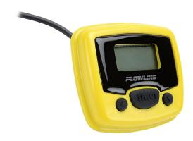
Flowline PodView general purpose digital indicator, polycarbonate, NEMA 4, IP65, 6ft (1.8m) 22AWG 4-conductor cable, panel mount. For use with Flowline EchoPod DL, DS and DX series ultrasonic level sensor with firmware V50.0 or later.
