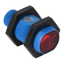
Contrinex photoelectric sensor, tubular, threaded, ABS plastic, diffuse with background suppression, 10-250mm sensing distance, complementary light-on/dark-on, PNP, teach-in button, 700 Hz switching frequency, 4-pin M12 quick-disconnect.
