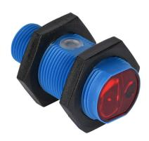
Contrinex photoelectric sensor, tubular, threaded, ABS plastic, diffuse with background suppression, 10-250mm sensing distance, complementary light-on/dark-on, NPN, teach-in button, 700 Hz switching frequency, 4-pin M12 quick-disconnect.
