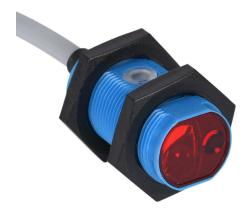
Contrinex photoelectric sensor, tubular, threaded, ABS plastic, diffuse with background suppression, 10-250mm sensing distance, complementary light-on/dark-on, PNP, teach-in button, 700 Hz switching frequency, 6.5ft/2m cable length, pigtail.
