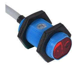
Contrinex photoelectric sensor, tubular, threaded, ABS plastic, diffuse with background suppression, 10-250mm sensing distance, complementary light-on/dark-on, NPN, teach-in button, 700 Hz switching frequency, 6.5ft/2m cable length, pigtail.
