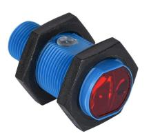
Contrinex photoelectric sensor, tubular, threaded, ABS plastic, diffuse with background suppression, 10-250mm sensing distance, complementary light-on/dark-on, PNP, potentiometer, 700 Hz switching frequency, 4-pin M12 quick-disconnect.
