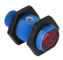
Contrinex photoelectric sensor, tubular, threaded, ABS plastic, diffuse with background suppression, 10-250mm sensing distance, complementary light-on/dark-on, NPN, potentiometer, 700 Hz switching frequency, 4-pin M12 quick-disconnect.
