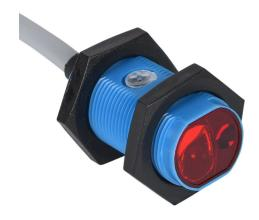
Contrinex photoelectric sensor, tubular, threaded, ABS plastic, diffuse with background suppression, 10-250mm sensing distance, complementary light-on/dark-on, PNP, potentiometer, 700 Hz switching frequency, 6.5ft/2m cable length, pigtail.
