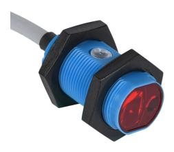
Contrinex photoelectric sensor, tubular, threaded, ABS plastic, diffuse with background suppression, 10-250mm sensing distance, complementary light-on/dark-on, NPN, potentiometer, 700 Hz switching frequency, 6.5ft/2m cable length, pigtail.
