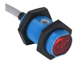
Contrinex photoelectric sensor, tubular, threaded, ABS plastic, diffuse with background suppression, 10-250mm sensing distance, complementary light-on/dark-on, NPN, potentiometer, 700 Hz switching frequency, 6.5ft/2m cable length, pigtail.
