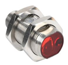
Contrinex photoelectric sensor, tubular, threaded, stainless steel, diffuse with background suppression, 10-250mm sensing distance, complementary light-on/dark-on, PNP, teach-in button, 700 Hz switching frequency, 4-pin M12 quick-disconnect.
