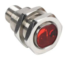
Contrinex photoelectric sensor, tubular, threaded, stainless steel, diffuse with background suppression, 10-250mm sensing distance, complementary light-on/dark-on, NPN, teach-in button, 700 Hz switching frequency, 4-pin M12 quick-disconnect.
