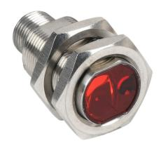
Contrinex photoelectric sensor, tubular, threaded, stainless steel, diffuse with background suppression, 10-250mm sensing distance, complementary light-on/dark-on, PNP, potentiometer, 700 Hz switching frequency, 4-pin M12 quick-disconnect.
