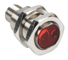
Contrinex photoelectric sensor, tubular, threaded, stainless steel, diffuse with background suppression, 10-250mm sensing distance, complementary light-on/dark-on, NPN, potentiometer, 700 Hz switching frequency, 4-pin M12 quick-disconnect.
