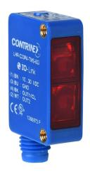
Contrinex photoelectric sensor, rectangular, diffuse with background suppression, 15-250mm sensing distance, complementary light-on/dark-on, PNP, teach-in button, 1000 Hz switching frequency, 4-pin M8 quick-disconnect.
