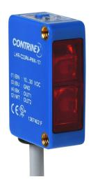
Contrinex photoelectric sensor, rectangular, diffuse with background suppression, 15-250mm sensing distance, complementary light-on/dark-on, NPN, potentiometer, 1000 Hz switching frequency, 6.5ft/2m cable length, pigtail.
