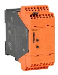
Dold safety relay, motor standstill monitoring, 0.2-4V, 2-channel, 24 VDC, (3) N.O. and (1) N.C. safety output(s), push-in cage clamp.
