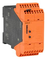
Dold safety relay, motor standstill monitoring, 0.2-4V, 2-channel, 115 VAC, (3) N.O. and (1) N.C. safety output(s), push-in cage clamp.
