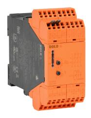
Dold safety relay, motor standstill monitoring, 20-400 mV, 2-channel, 115 VAC, (3) N.O. and (1) N.C. safety output(s), push-in cage clamp.
