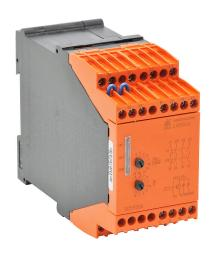
Dold safety relay, motor standstill monitoring, 20-400 mV, 2-channel, 24 VDC, (3) N.O. and (1) N.C. safety output(s), fixed screw terminals.
