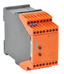
Dold safety relay, motor standstill monitoring, 0.2-4V, 2-channel, 115 VAC, (3) N.O. and (1) N.C. safety output(s), fixed screw terminals.
